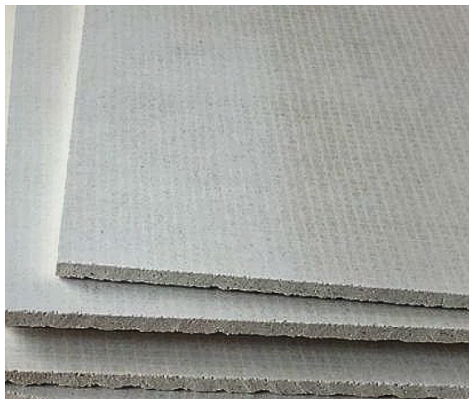
Boards cut to size and ready for bedding in adhesive.
